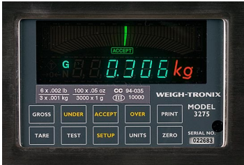
Fan graph displays showing underweight indication and target weight indication
