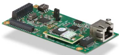
Wireless Internal Card 802.11 b/g Wireless
