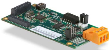
Analog Output Card 0-10 VDC and 4-20 mA.
