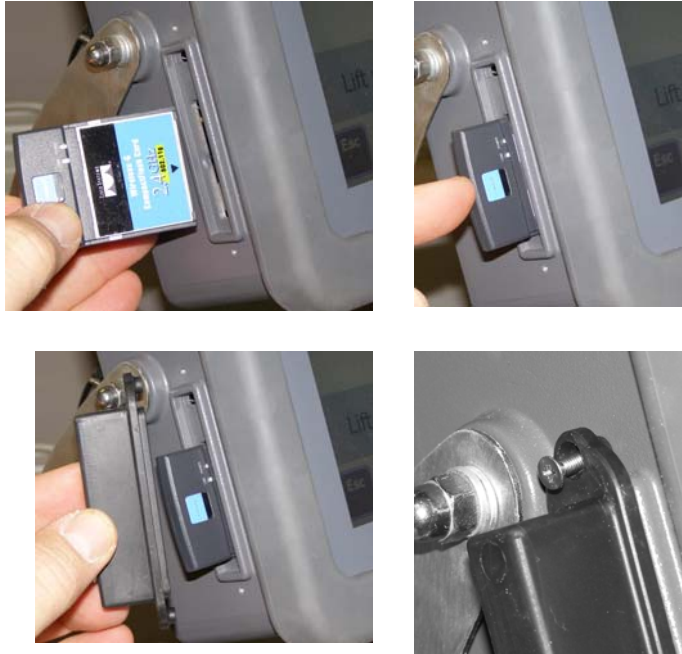
Figure 10.1 Installing the Compact Flash radio
