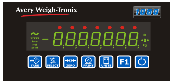
Figure 3.1 Model 1080 front panel
