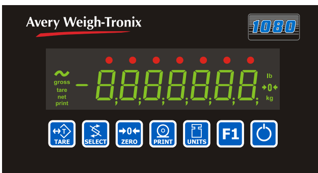
Figure 2.1 Front panel of the 1080 indicator
