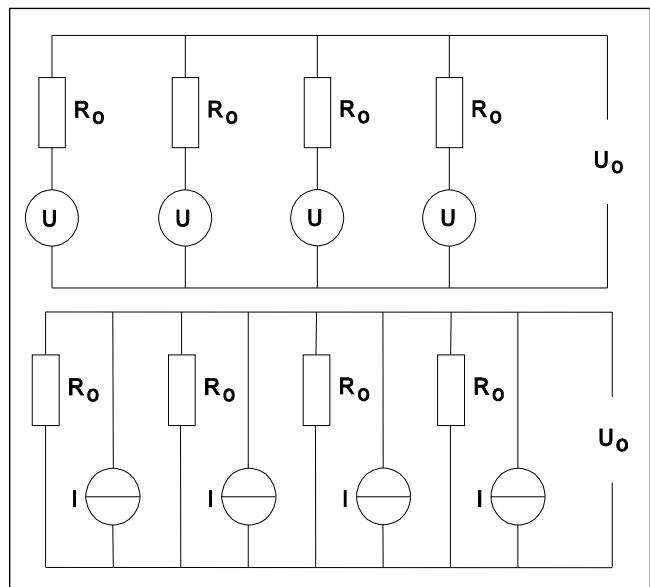
as a current source, driving current through the parallel combination of the load cell source impedances, where  $I = U / R_o$ .
