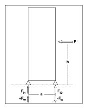
$F_l$ = Force on load cell  $F_w$ = Force caused by wind force
