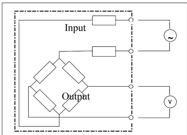
zero output changes per time period are most likely undergoing a change in the strain gauge resistance because of chemical or moisture intrusion. However, in this case the insulation resistance and/or the bridge integrity will also be compromised.
