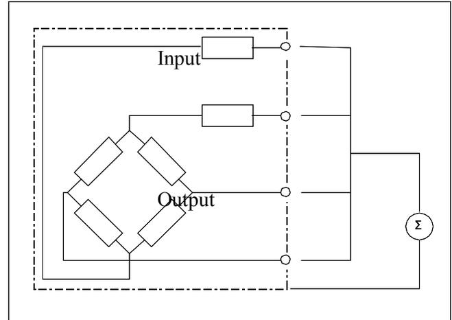
load cell or cable. Extremely low values ( $\leq 1k \Omega$ ) indicate a short circuit rather than moisture ingress.
